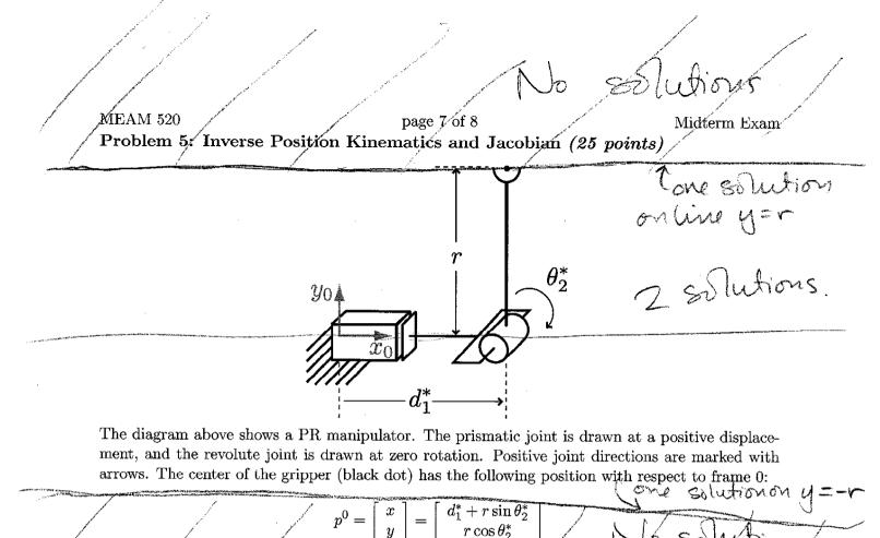
a. Assume this robot has no joint limits and will not collide with itself in any configuration. Given a desired position of the end effector  $[x \ y]^T$ , find all possible solutions to this robot's planar inverse position kinematics. In addition to providing equations for  $d_1^*$  and  $\theta_2^*$ , please state how many solutions there are to the inverse kinematics problem, and explain how the number of solutions depends on the desired position. (10 points)
