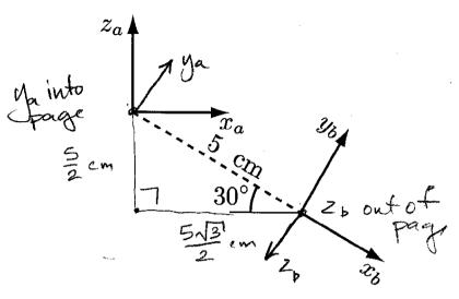
a. What is  $H_b^a$ , the homogeneous transformation representing the position and orientation of frame b in frame a? (10 points)
