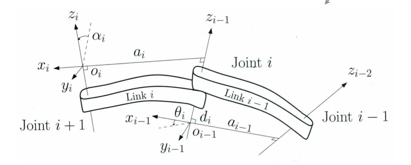
The **Denavit-Hartenberg convention** defines four parameters and some rules to help characterize arbitrary kinematic chains
