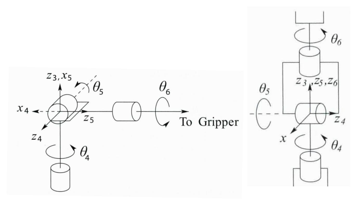
Note: Spherical wrist in Figure 3.8 is drawn with  $\theta_5 = -90^\circ$
