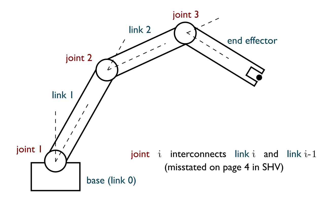
In a serial kinematic chain, each intermediate link is connected to two others
