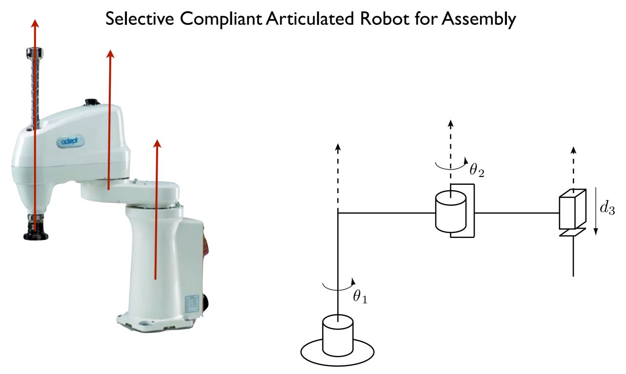
Introduced in 1979, The SCARA manipulator design revolutionized the assembly of small electronics
