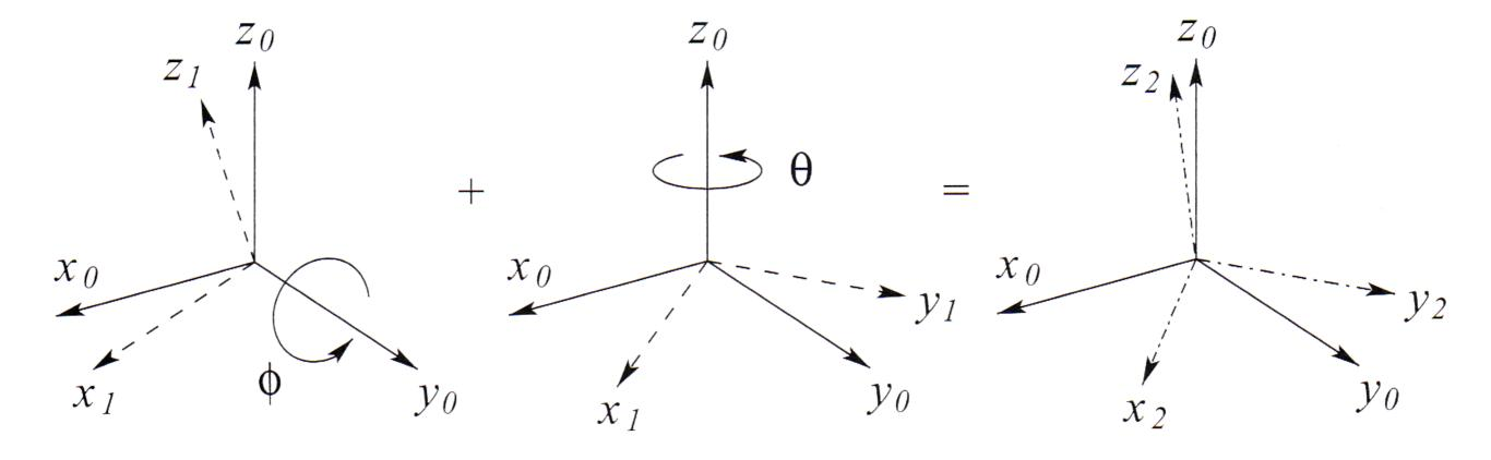
the result of a successive rotation about a fixed frame can be found by **pre-multiplying** by the corresponding rotation matrix
