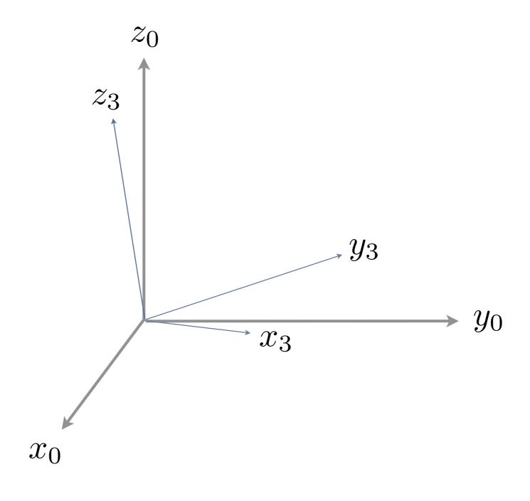
step I:rotate by  $\phi$  about  $z_0$
