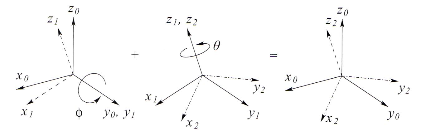
the result of a successive rotation about the current (intermediate) frame can be found by **post-multiplying** by the corresponding rotation matrix
