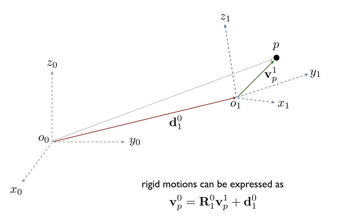
a **homogeneous transformation** is a matrix representation of rigid motion, defined as
