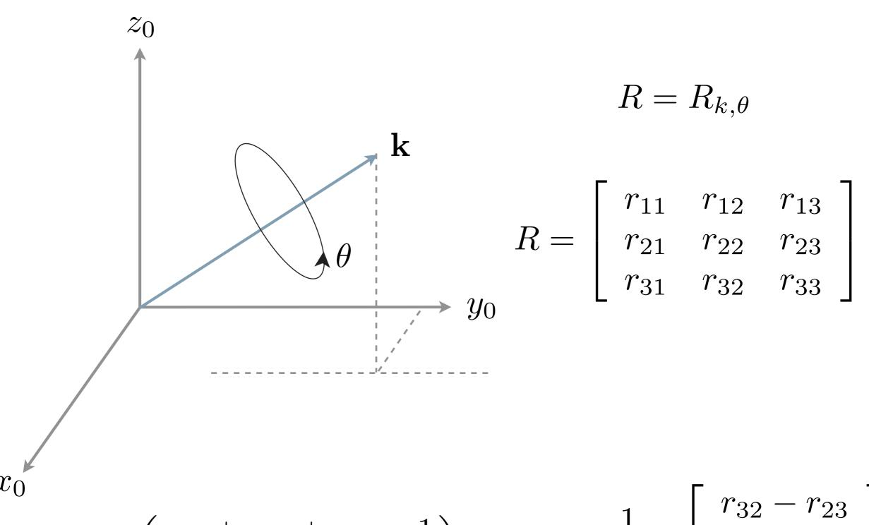
$$\theta = \cos^{-1}\left(\frac{r_{11} + r_{22} + r_{33} - 1}{2}\right) \qquad k = \frac{1}{2\sin\theta} \begin{bmatrix} r_{32} - r_{23} \\ r_{13} - r_{31} \\ r_{21} - r_{12} \end{bmatrix}$$
