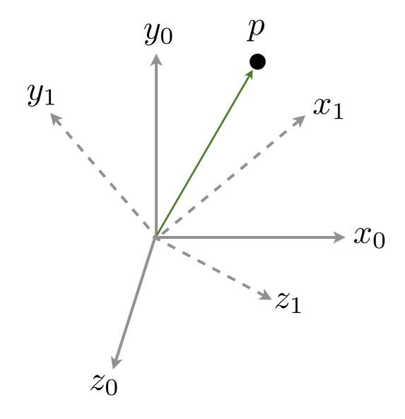
For pure coordinate rotation, a point in frame I can be expressed in frame 0 using the rotation matrix
