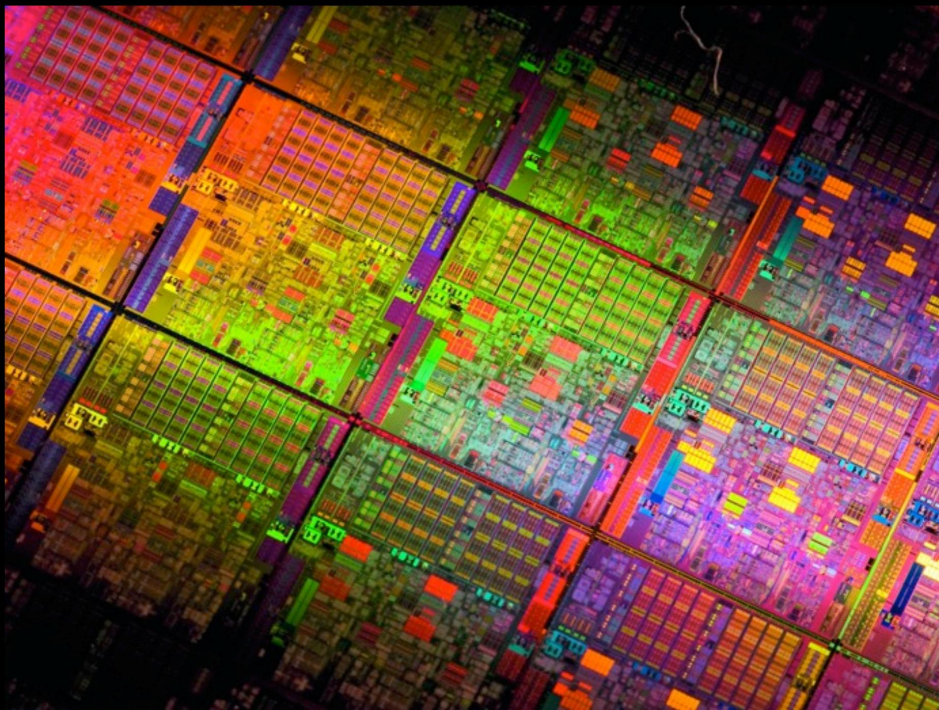
(Intel Gulftown Six-core processor - 1.17B transistors)
