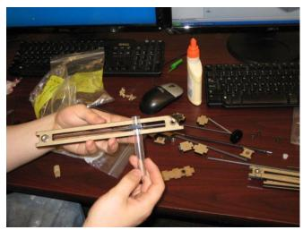
**Friction:** Due to excessive friction caused by the acrylic gliding on the aluminum rods, we encountered a problem with the original design for the part that would hold the writing utensil with the sliding arms. We had to redesign a simpler contraption that would smoothly glide in both directions along the moving arms.
