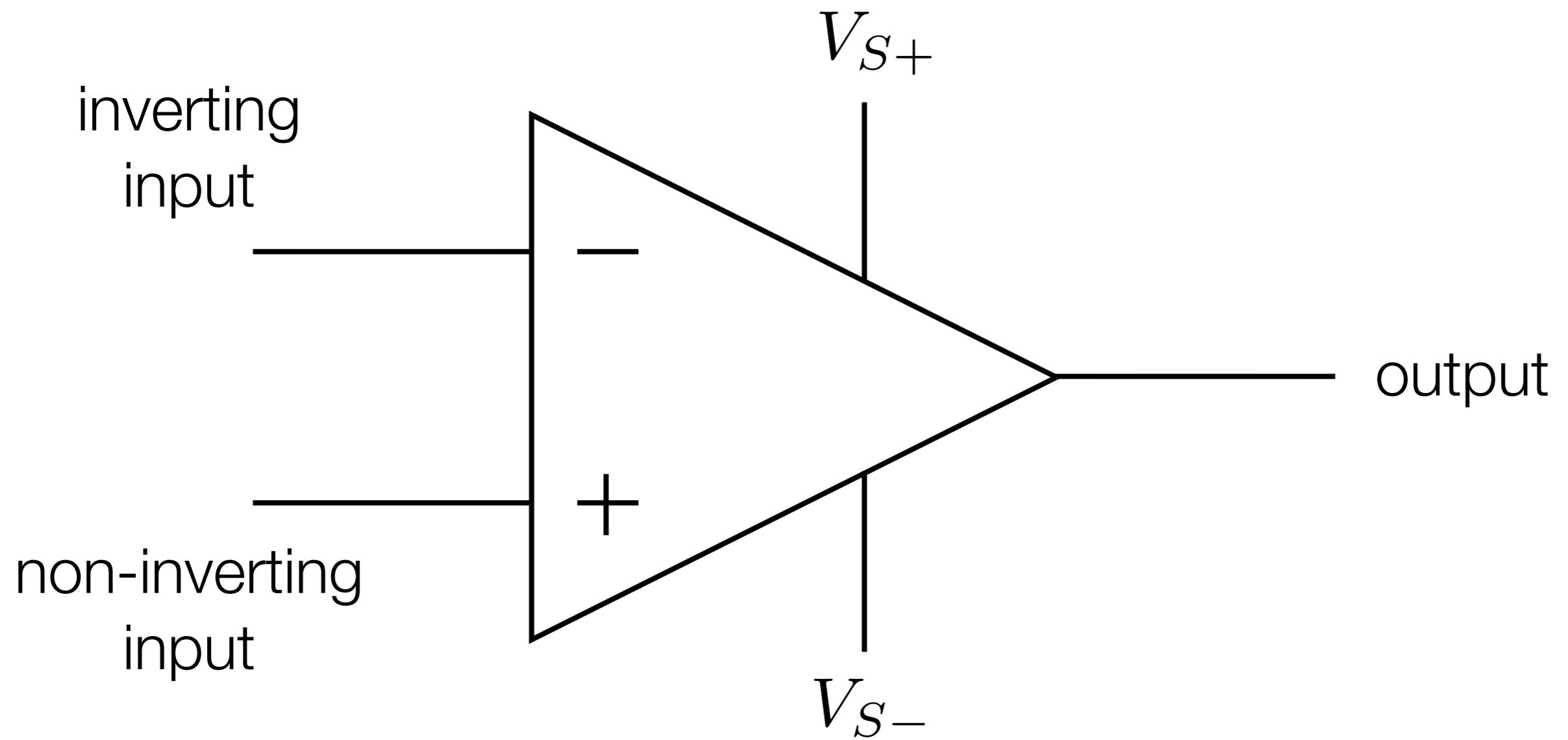
output = amplified difference between inputs
