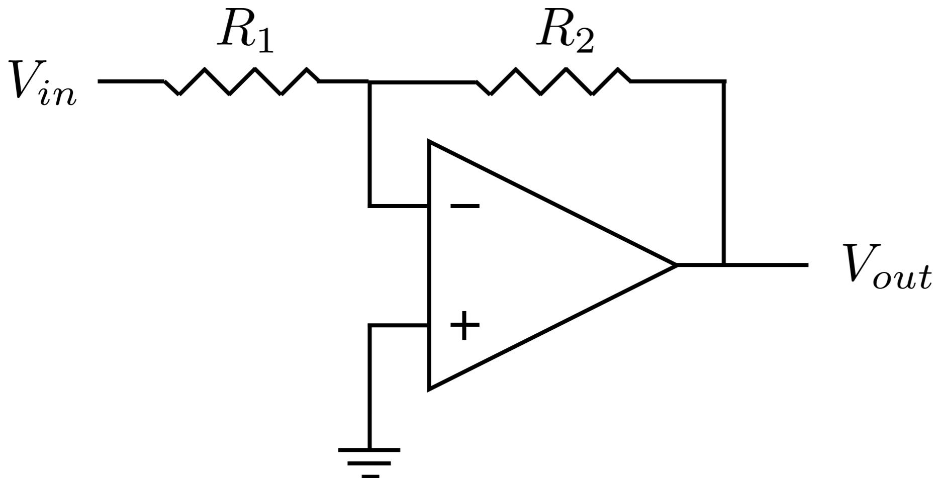
$$\frac{V_{out}}{V_{in}} = -\frac{R_2}{R_1}$$
