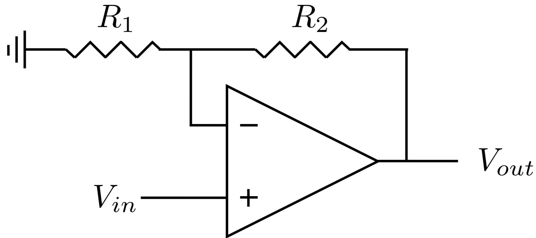
$$\frac{V_{out}}{V_{in}} = 1 + \frac{R_2}{R_1}$$
