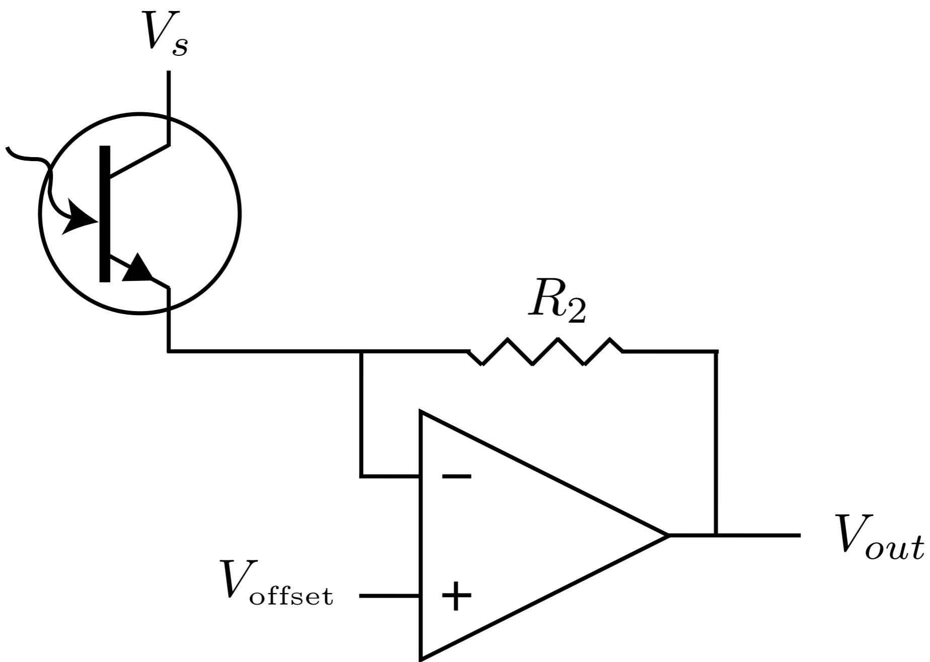
$$V_{\text{out}} = V_{\text{offset}} - R_2 \ i_{\text{photo}}$$
