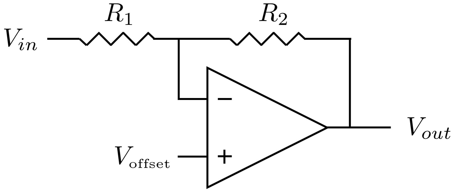
$$V_{out} = V_{offset} \left( 1 + \frac{R_2}{R_1} \right) - V_i \frac{R_2}{R_1}$$
