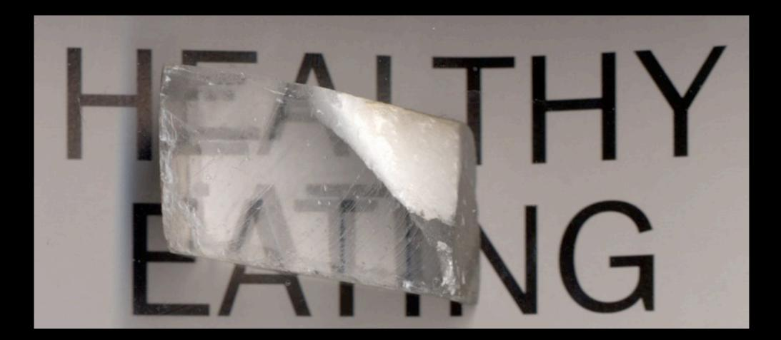
A MATERIAL PROPERTY THAT SPLITS A RAY OF LIGHT INTO TWO SEPARATE RAYS
