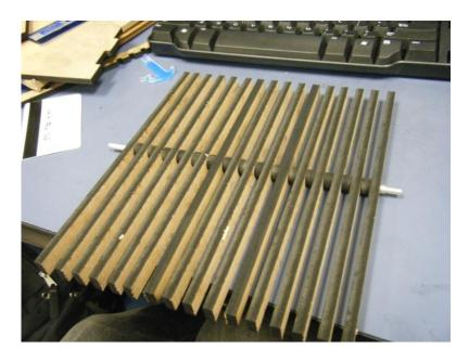
Starting to come together: The way the automata was modeled allowed us to create several iterations of a single part to create the main components of our project. The waves were cut with the hole slightly off-center so that they would be unbalanced on the rod and thus not lose contact with the top of the cams. The thickness of the material and the length of the model was planned so that we could use the same material for our parts as well as our spacers between them.
