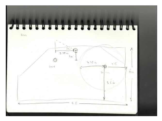
*Calculations*: First, we determined what we thought would be a reasonable angle for the desired maximum height of the waves. Then, we had to determine the placement of the cam-rod and central axle, as well as the size of the cams, that would give us the desired height. We also had to determine the placement of the dolphin-rod so that the dolphins would come above the waves at some point during their rotation, but not collide with the central axle.
