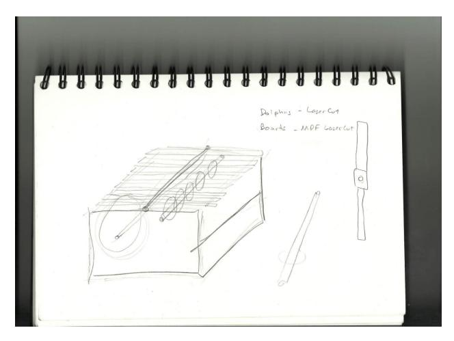
*Method*: Cams may be held in place through glue/rubber stoppers/screws/spacers. Other considerations discussed included attaching the rods to the gears and attaching the crank to one of the gears. Gears are to be laser cut, as metal tools at our disposal are not precise enough.
