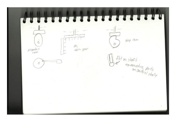
*Mechanisms*: The different motions we could produce by using different mechanisms were brainstormed. Some of these mechanisms were sketched above. Some possible mechanisms discussed included different types of cams, pistons, bevel gears, and crank sliders.
