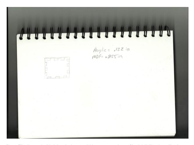
*Press Fits*: It was decided that the box would be constructed out of both MDF and acrylic pieces. The acrylic pieces would go on the side to display the mechanisms that drove the automata. The thicknesses of the materials were also recorded so that press fits could be accurately modeled.
