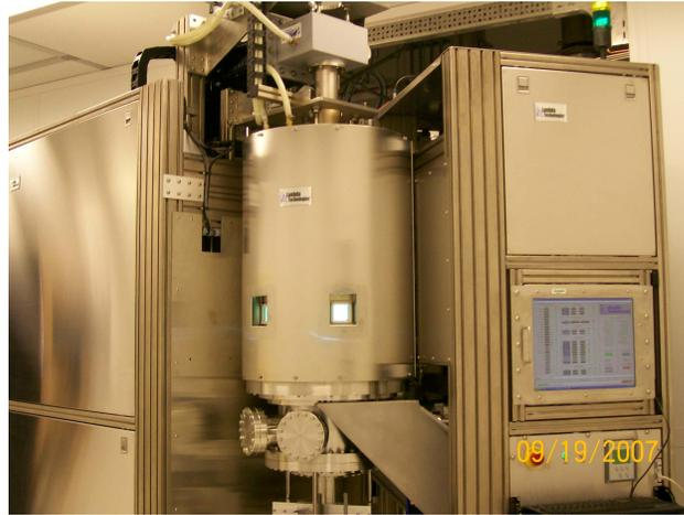
Figure 1. 915 MHz large area MPCVD system in operation in the clean room at the Center for Nanoscale Materials, ANL.
