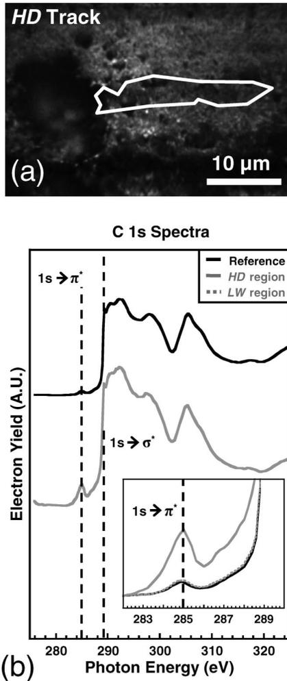
FIG. 2. (a) X-PEEM image at 289 eV inside the *HD* track. (b) C 1s spectra, offset for clarity. The top spectrum (black line) is a reference taken far from the wear track, and the bottom spectrum (gray line) is from the region drawn in (a). Inset: magnified plot of the spectra from (b) and a spectrum from track *LW*, in the  $1s \rightarrow \pi^*$  region.
