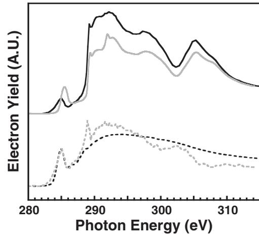
FIG. 3. A comparison of NEXAFS spectra. Top: experimental data from the most heavily worn region of the *HD* wear track (solid black line) and a simulation for one monolayer of graphite on UNCD (solid gray line). Bottom: spectrum from hydrogenated amorphous carbon (dashed black line) and subtraction of an unworn UNCD spectrum from the *HD* track spectrum (dashed gray line).
