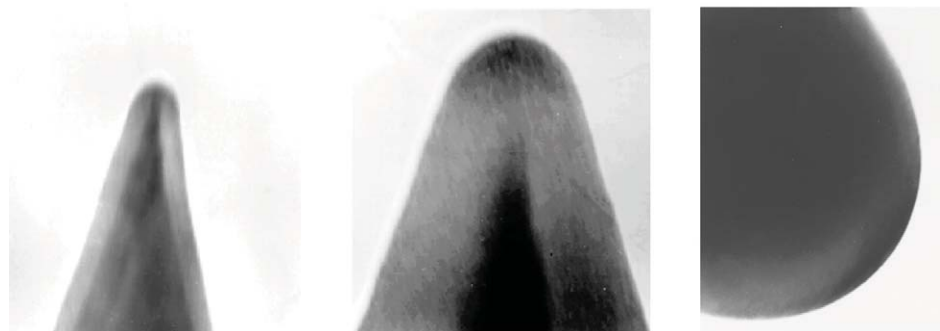
Fig. 11 Transmission electron micrographs of three different tips with spherical apices prepared using electron beam induced decomposition inside the TEM. (Reproduced with permission from 39 . © 1997 American Physical Society.)
