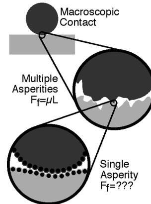
Fig. 1. The typical surface roughness of macroscopic interfaces ensures a complex multitude of contact points (asperities). A scanning force microscope provides a well-defined single asperity contact (the tip) where interaction forces can be precisely measured with nanometer/atomic resolution. Friction deviates from macroscopic behavior at this scale.
