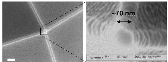
Fig. 4. SEM images of a pyramidal AFM tip coated with DLC. The apparent roughness is due to the pre-existing texture of the silicon nitride tip. At left, scale bar = 200 nm.
