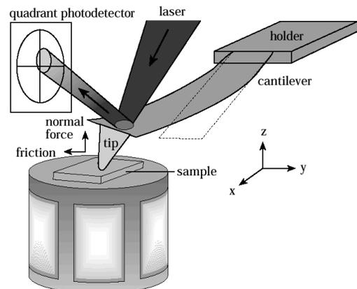
Fig. 2. Schematic of the typical AFM set-up. The tip is in contact with a sample surface. A laser beam is focused on the back of the cantilever and reflects into a four-quadrant photodetector. Normal forces deflect the cantilever up or down, lateral forces twist the cantilever left and right. These deflections are simultaneously and independently measured by monitoring the deflection of the reflected laser beam.
