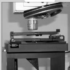
MultiView 2000™ - The only tip or sample scanning SPM/NSOM
