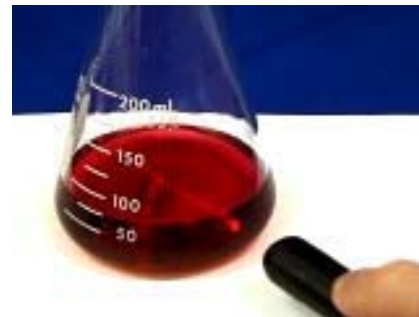
Figure 4. A reddish suspension of gold nanoparticles is produced by reduction of a gold (III) salt. The presence of the gold colloid can be detected by the scattering of a laser beam by the nanoparticles. 29
